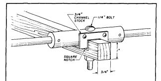
fig. 4. A short piece of square channel stock locks center block firmly in place on support mast. A 1/4-inch bolt holds the antenna in place.
