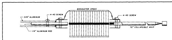
fig. 3. End sections slip into 3/8-inch elements and are locked in place with a No. 4-40 screw. Solder lugs provide electrical connections for loading coils.
