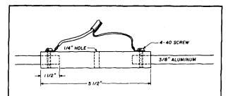
fig. 2. The 3/8-inch elements slip into the center block, and lock in place with No. 4-40 screws. Only one element need be removed to break down and transport the antenna.
