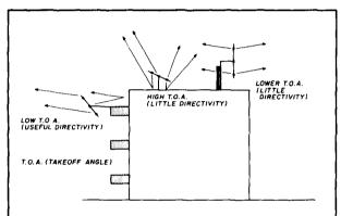
fig. 5. Conductive surfaces on buildings may be an advantage or disadvantage, depending on how you use them. On 20 meters, placing a horizontal dipole near the surface of a conductive roof may produce poorer results than mounting vertically, or mounting off to one side of the building!
